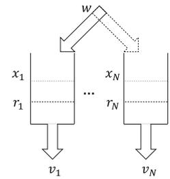
ics  $\dot{x}_i = -v_i$ , for a real constant  $v_i \geq 0$ . One of the tanks is filled from an external inlet at some constant flow rate  $w$ , so it has dynamics  $\dot{x}_i = w - v_i$ , for a real constant  $w \geq 0$ . In our variant, the volume lost by each tank simply vanishes and does not move from one tank to another. This benchmark class is qualitatively different than either the navigation or satellite benchmarks, as the discrete state space may be small.
