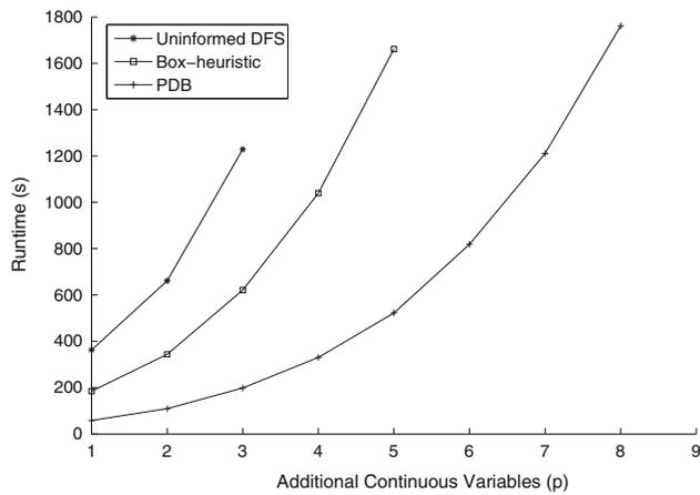
**Fig. 12** Navigation benchmark with additive vanishing perturbation for  $1 \leq p \leq 8$  with the same discrete structure as instance 1 (i. e., all else constant except the number of additive perturbation terms). The total number of continuous variables is  $n = 4 + p$
