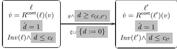
**Fig. 3.** DTR( $\mathcal{H}, dtb$ ), the dwell time refinement of  $\mathcal{H}$  for a given family of dwell time bounds  $dtb$  valid for  $\mathcal{H}$ , is obtained from  $\mathcal{H}$  by a transformation that adds the highlighted items; among those, the dwell time constraints  $d \leq c_\ell$  and  $d \geq c_{(\ell, \ell')}$
