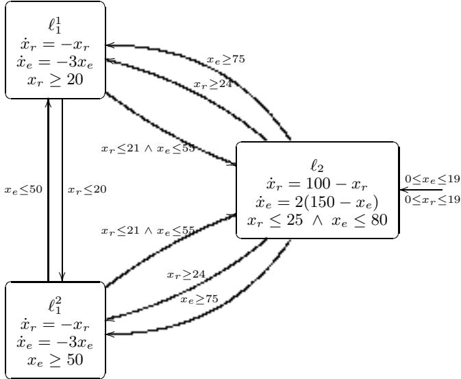
**Fig. 1.** Example hybrid system, modeling a temperature controller with one internal engine. The temperature of the plant is controlled through a thermostat which turns the engine off and on, depending on the temperature of the room (modeled by the continuous variable  $x_r$ ) and the temperature of the engine (modeled by the continuous variable  $x_e$ ). We model the mode ‘off’ by the two locations  $\ell_1^1$  and  $\ell_1^2$ , and the mode ‘on’ by the location  $\ell_2$ .
